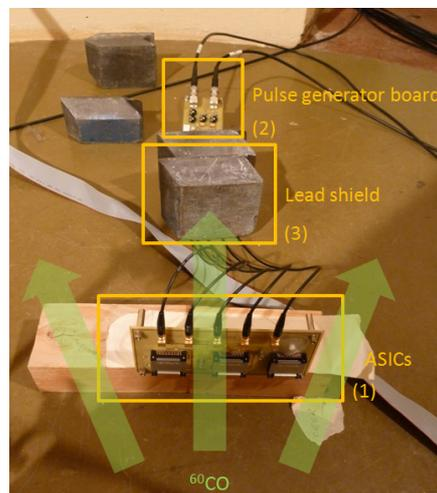
Fig. 5. Irradiated ASICs PCB with its power-supply and input stimuli PCB protected by a lead shield.
