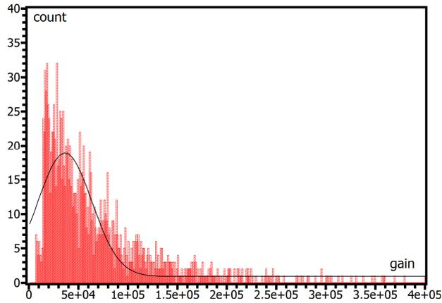
Fig. 4. Measured MCP pulse gain distribution at 2650 V due to charges of an MCP illuminated by an electron beam.
