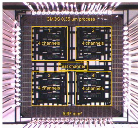
Fig. 3. Die photograph of the 16 channel readout circuit and a test channel.
