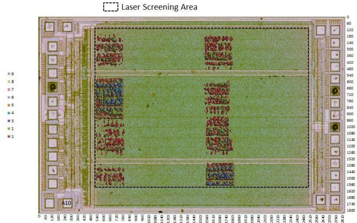
Fig. 7. Representation of the Alliance cost SRAM screening map. Sensitive memory cell blocks have been detected
