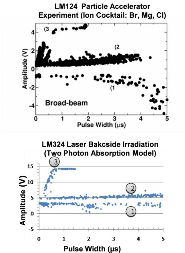
Fig. 4. Comparison between heavy ions in a particle accelerator [8] and laser irradiation in the UCM laser facility.
