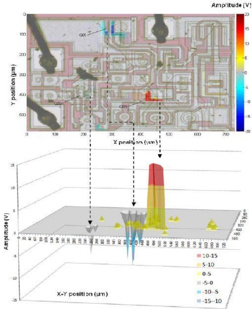
Fig. 6 Sensitive maps after a complete LASER scan over the LM124. 2D view (up) and 3D view (bottom) data representation.
