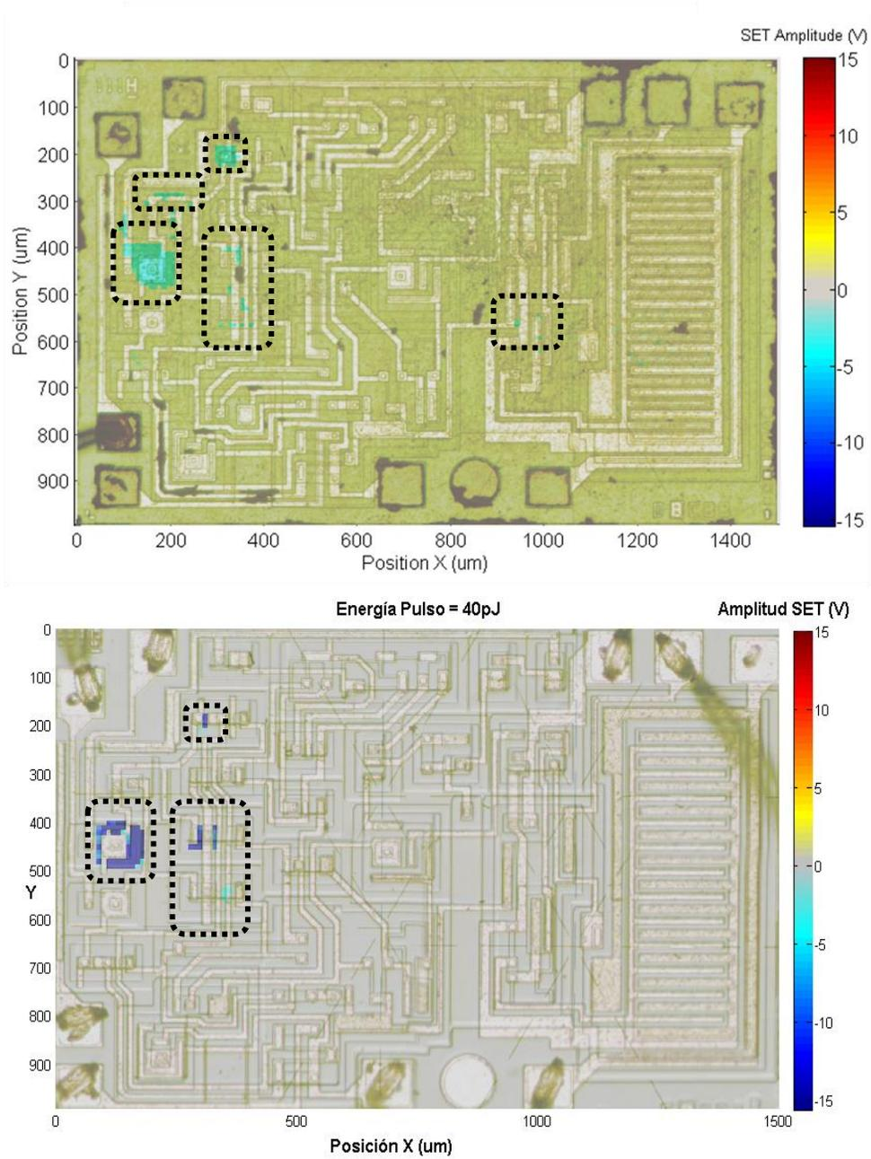
Fig. 5 . Comparison of back-side (up) and front-side (bottom) laser test of the LM111 with TPA. Wavelength = 1300 nm, pulse energy = 50 pJ, pulse width= 80 fs, spot size = 1.5  $\mu\text{m}^2$ .
