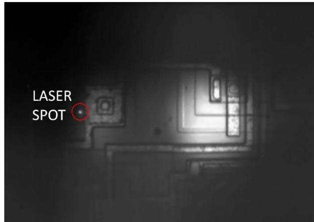
Fig. 2. Microphotography of the LM124 integrated circuit. LASER spot is located in one of the transistors at the input stage.
