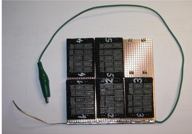
Fig. 4 Test specimens mounted on the plate
