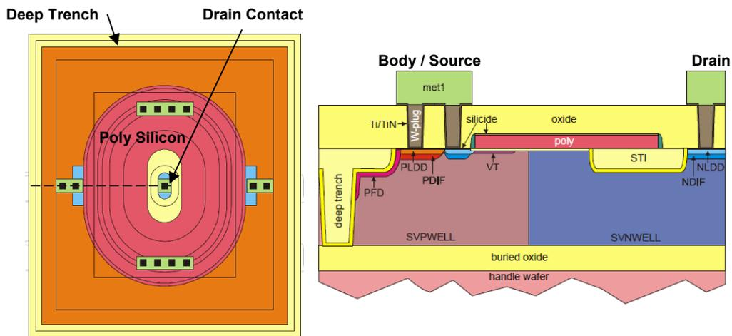
Fig. 1 Typical top-view (left) and the cross-section (right) of a DMOS device of TFSMART2 technology which is scalable in the width direction. Dashed line shown on the left depicts the device cross-section on the right sketch.
