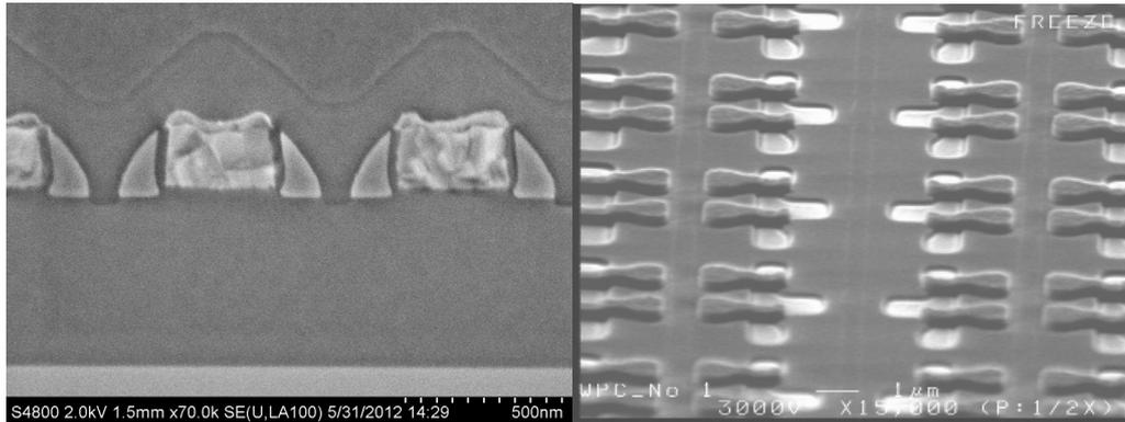
Fig. 3 Low voltage (3.3V) gate array and the cross-sections 350nm poly-gates of TFSMART2
