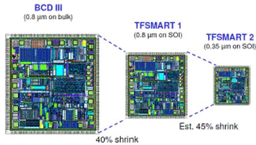
Fig. 2 Estimated shrink that can be achieved with 0.35μm SOI technology
