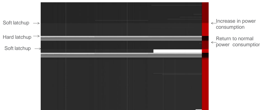
Figure 9: Example of SEFT's, soft and hard latch-ups detected by the EGSE during irradiation. The red vertical line is a measure for the FPA current.
