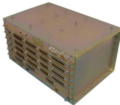
Figure 3 : BepiColombo RIU Engineering Model Showing a Large Number of Analogue I/O Connections for Environmental Sensors.
